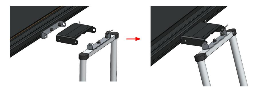
NOTE: The telescopic ladder must be fully locked in it's extended position for this bracket to work correctly. The ladder must be grounded, taking the weight of the user. The ladder must not have the weight HANGING on the bracket
